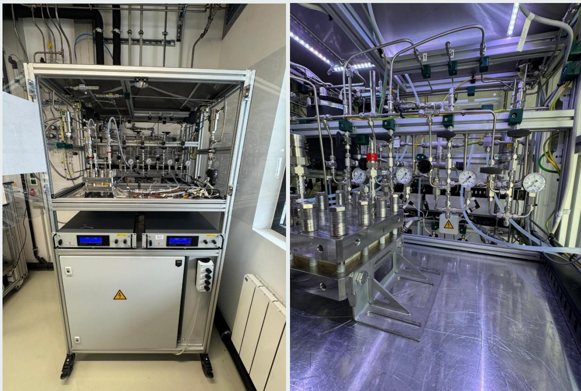
Figure 1: PEM Single cell testbench L.I.S.A integrated into the state-of-the-art testing infrastructure at HyCentA
