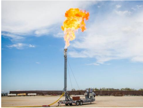
Fig. 1 Mobile flare for natural gas pipeline operation [1]
