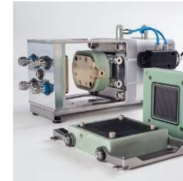
Testzellensystem qCf FC25/100: https://balticfuelcells.de/htmldocs/de/testgeraete_qcf-fc25.shtml
