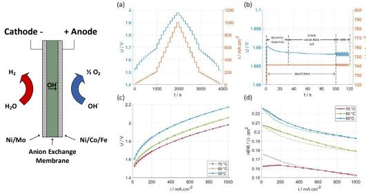
Schematic illustration of AEM water electrolysis (left) and measurement data from in-situ characterization of electrodes (right); Source: HyCentA
